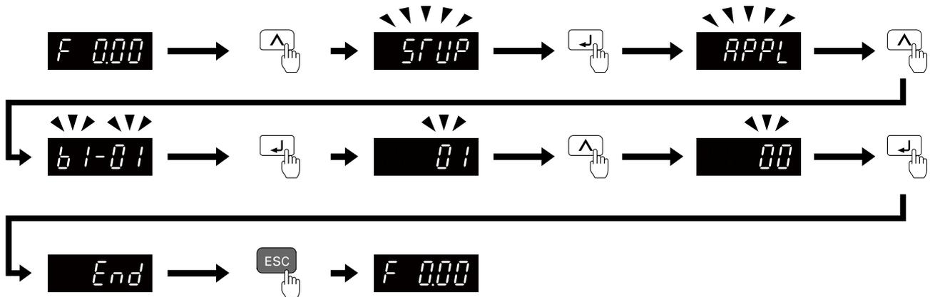
Figure 4.18 Set and View Quick Setup Parameters
