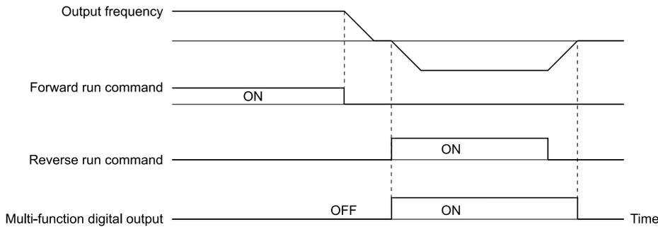
Figure 12.87 Reverse Operation Output Time Chart
