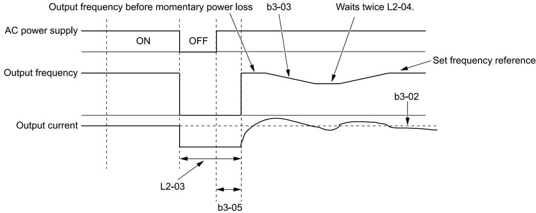
**Figure 12.22 Current Detection 2 after Momentary Power Loss**
