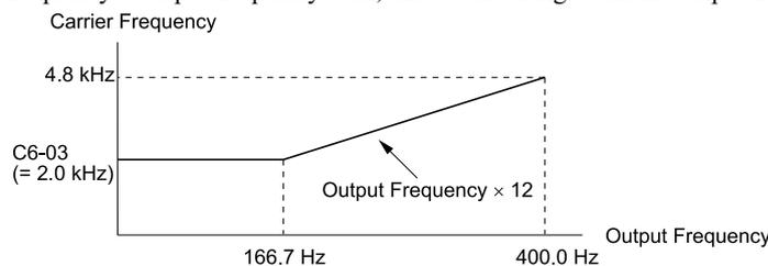
Figure 12.48 Carrier Frequency when C6-03 = 2.0 kHz, E1-04 = 400.0 Hz
