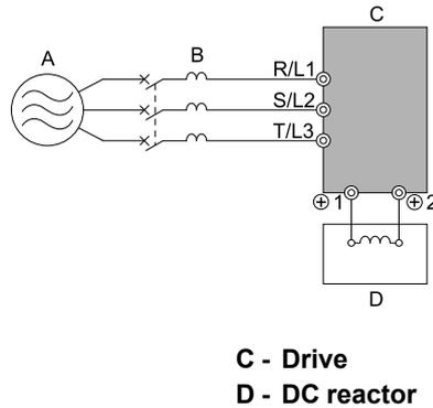
Figure 3.59 DC Reactor Connection Example
