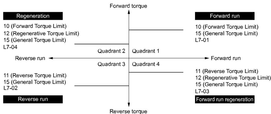
Figure 12.130 Torque Limits and Analog Input Setting Parameters
