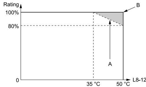
**A - L8-35 = 3 [External Heatsink] (default setting)**      **B - L8-35 = 0 [IP20/UL Open Type] (0.5 m/s of airflow around the drive is necessary)**
