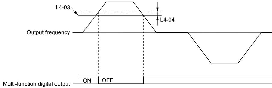
Figure 12.85 Example of Frequency Detection 3 (value of L4-03 Is Positive)
