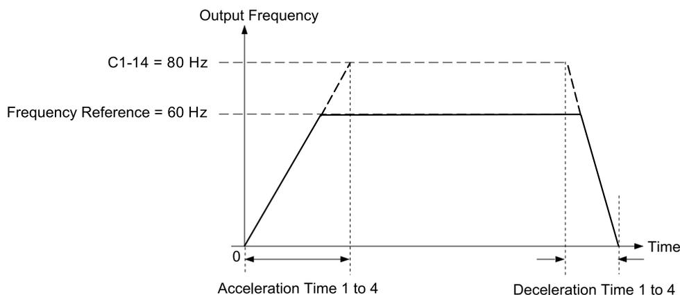
**Figure 12.40 Example 3: Acceleration/Deceleration Rate (When C1-14 = 80 Hz, E1-04 = 60 Hz, and the Frequency Reference is 60 Hz)**
