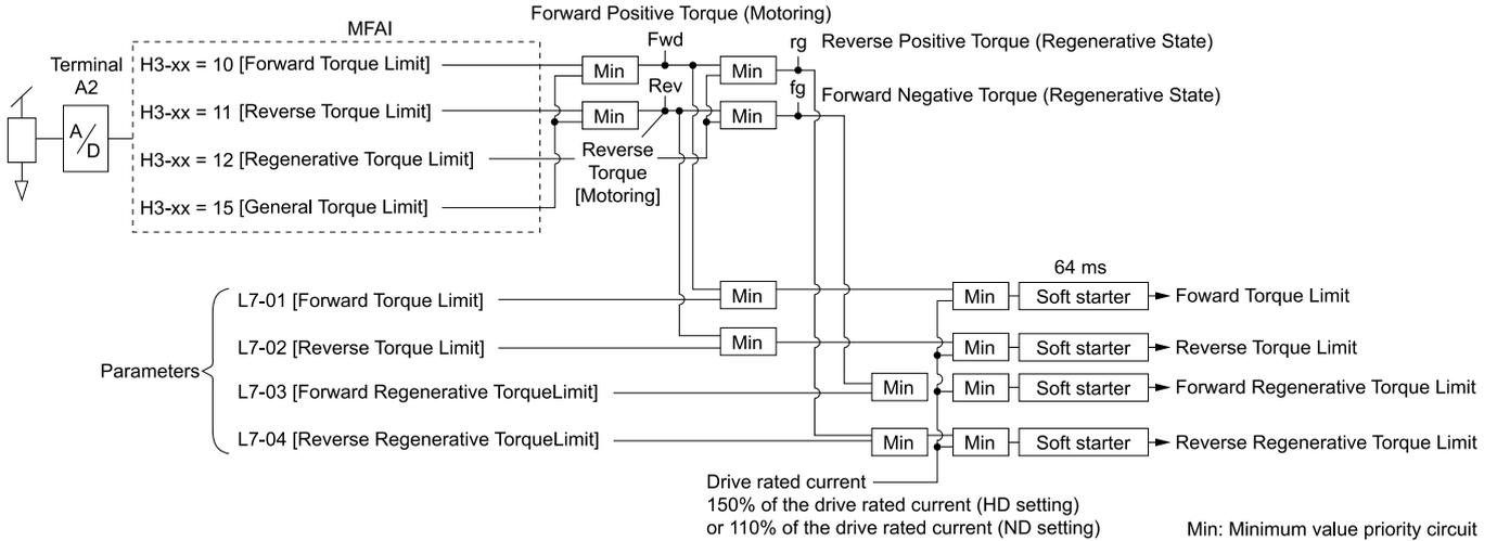
Figure 12.97 Torque Limits from Parameters and Analog Inputs
