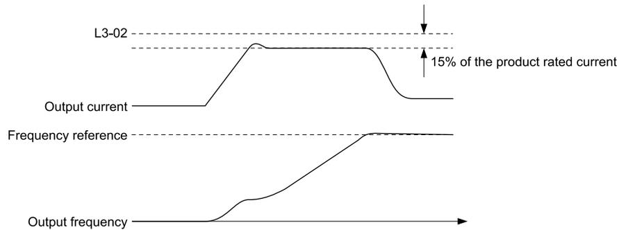
Figure 12.121 Current Limit Acceleration
