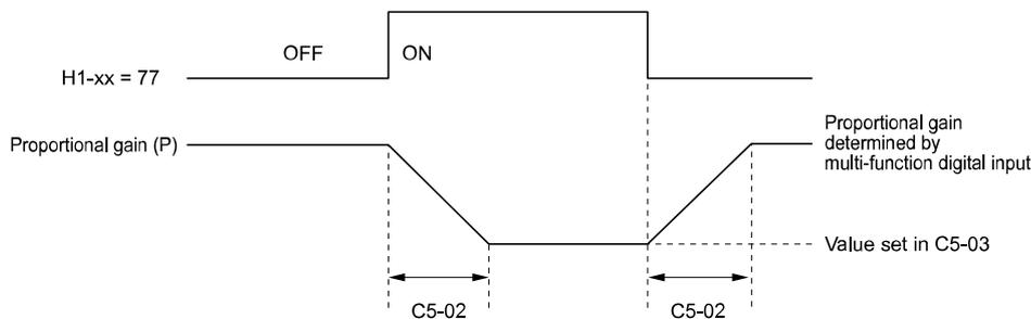
Figure 12.46 Proportional Gain through Multi-function Digital Input Switch
