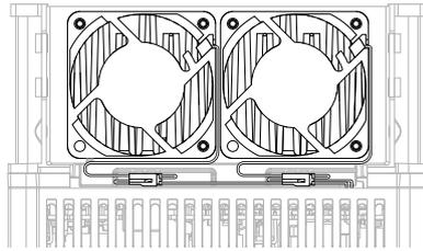
**Figure 8.6 Put the Connector in the Recess**
