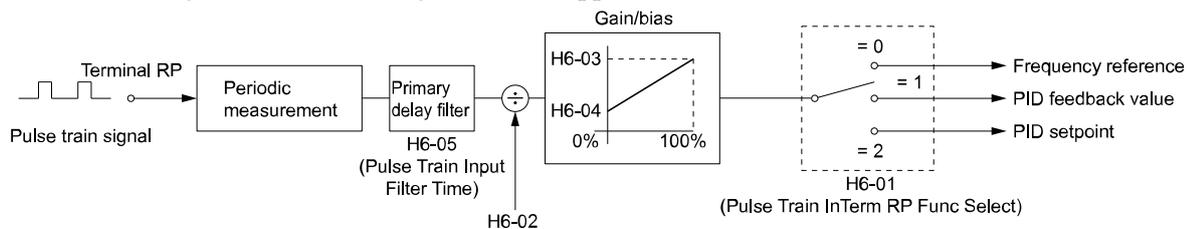
Figure 12.101 Pulse Train Input Block Diagram
