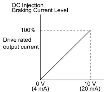
Figure 12.94 DC Injection Braking Current through Analog Input
