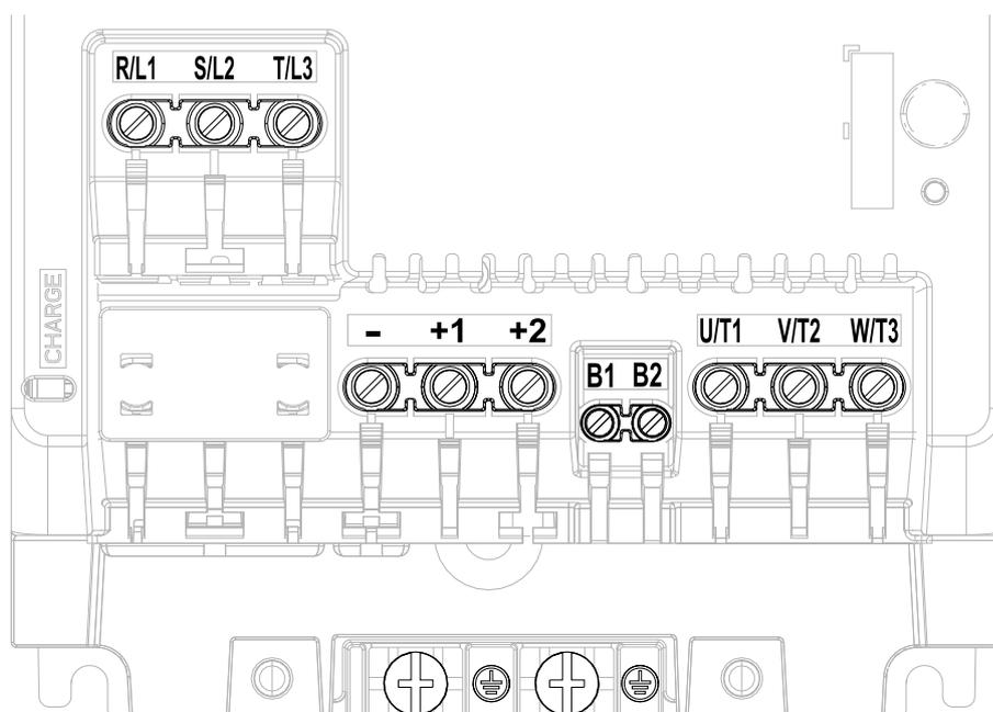
Figure 3.23 Configuration of Main Circuit Terminal Block (Three-Phase, With a Built-in EMC Filter)
