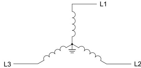
**Figure 5.7 Symmetric Grounding**
