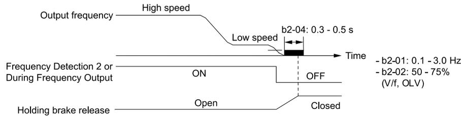
Figure 12.6 DC Injection Braking at Stop Function
