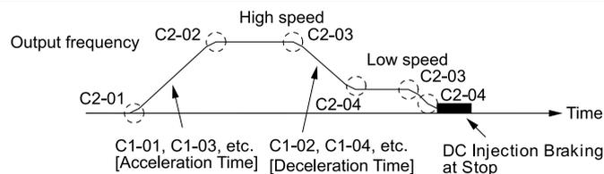
Figure 12.4 S-curve Characteristics, Accel &amp; Decel Time
