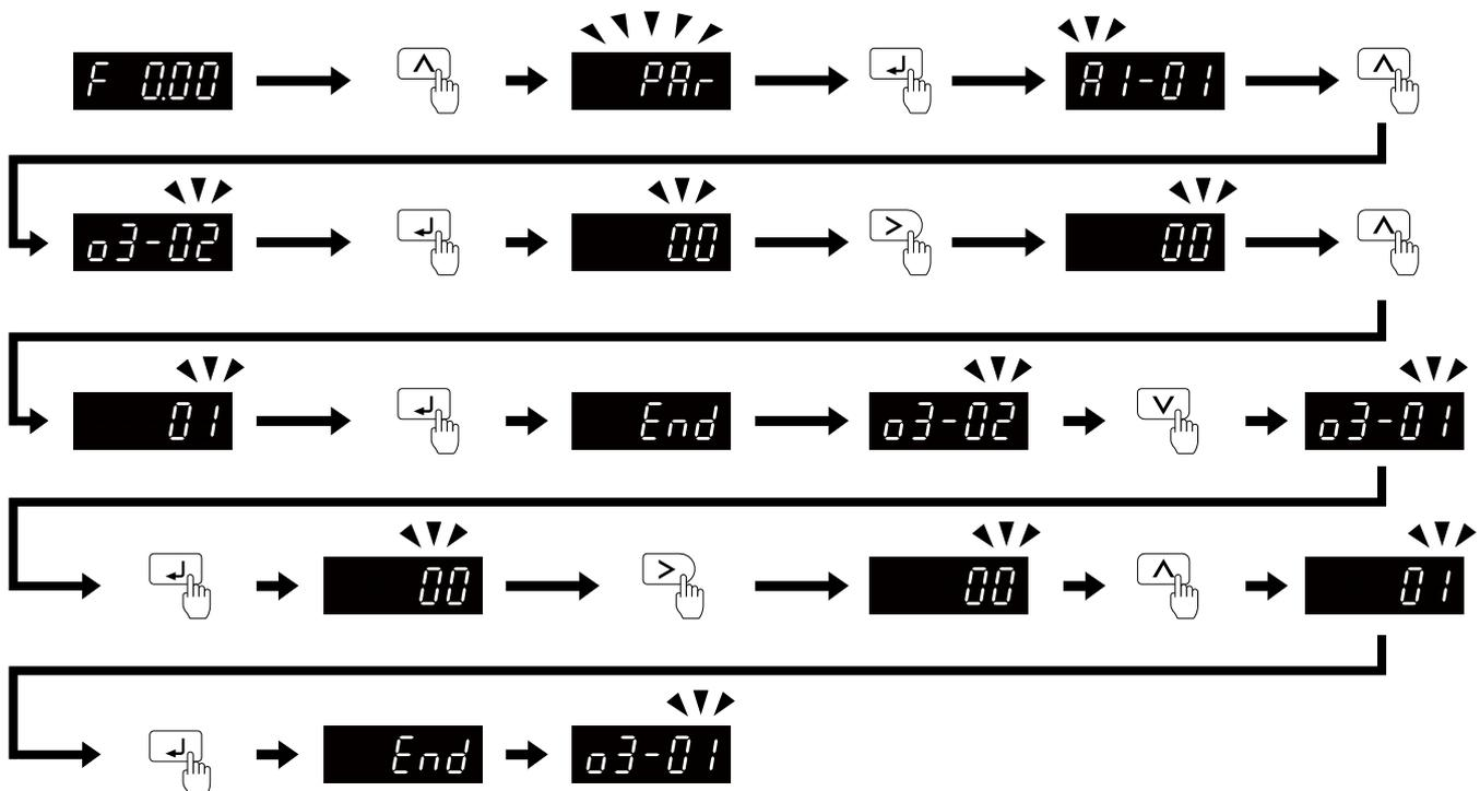
Figure 4.20 How to Save Backed-up Parameters
