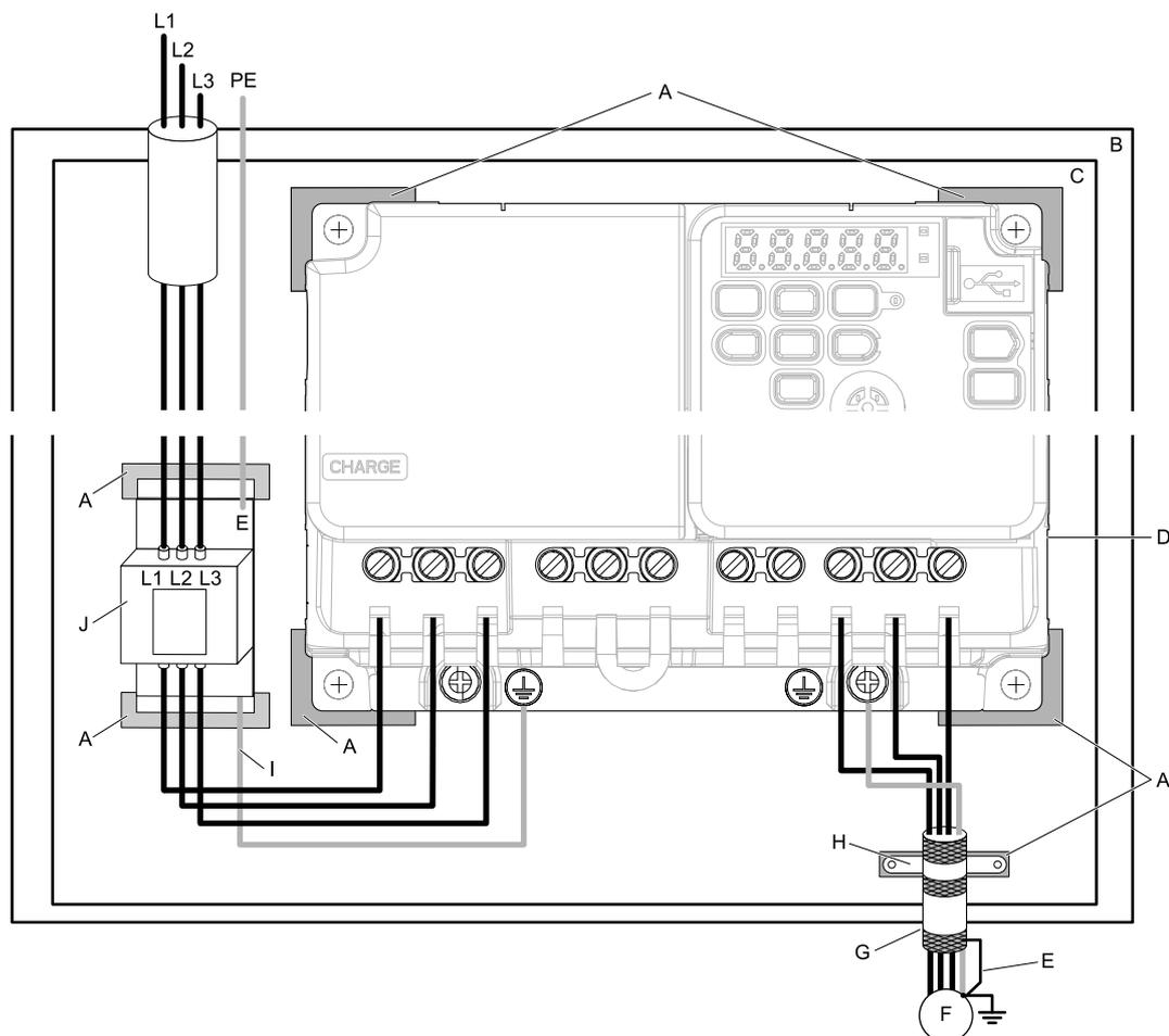
A - Grounding surface (Remove any paint or sealant.)
