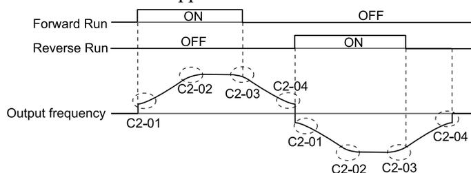
**Figure 12.41 S-Curve Timing Diagram - Forward/Reverse Operation**
