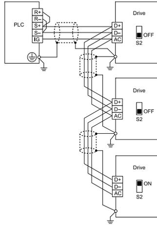
Figure 6.4 Wiring Diagram for More than One Drive
