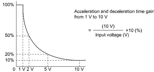
Figure 12.93 Acceleration/Deceleration Time Gain through Analog Input
