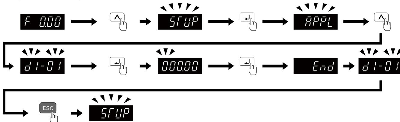
Figure 4.6 Parameters in General-Purpose Setup Mode
