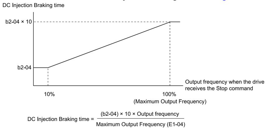
**Figure 12.13 DC Injection Braking Time and Output Frequency**
