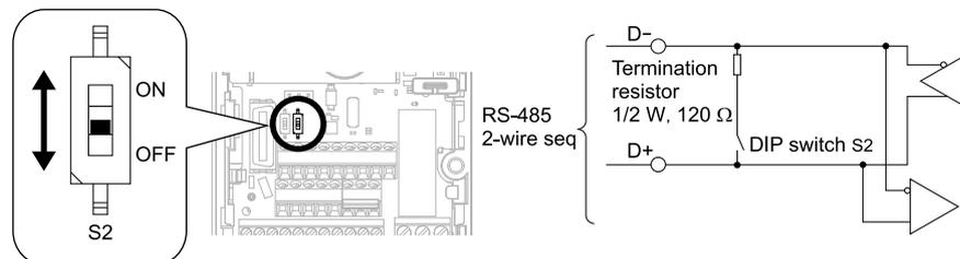
**Figure 6.3 MEMOBUS/Modbus Communication Terminal and DIP Switch S2**
