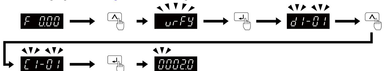
Figure 4.10 Verify and Set the Changed Parameters
