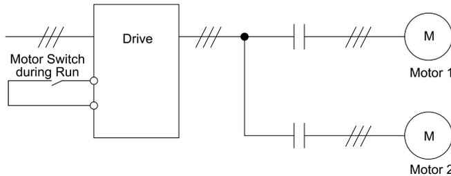
When you select motor 2, the drive will switch to motor 2 parameters.
