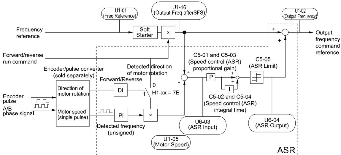
Figure 12.102 Simple Closed Loop Speed Control Block Diagram
