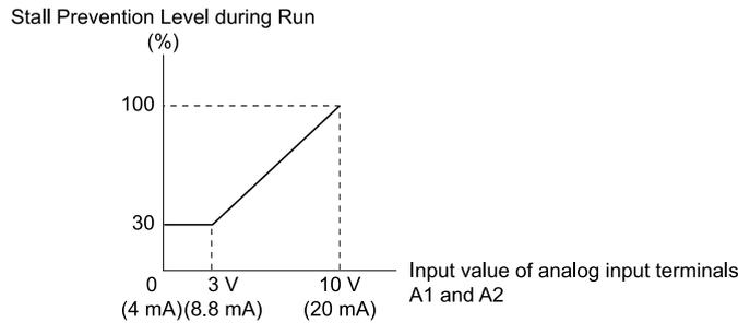
Figure 12.95 Stall Prevention Level during Run with Analog Input
