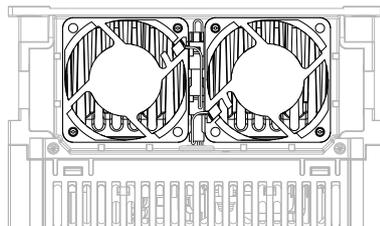
**Figure 8.7 Put the Connector in Between the Fans**
