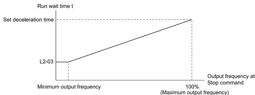
Figure 12.15 Run Wait Time and Output Frequency
