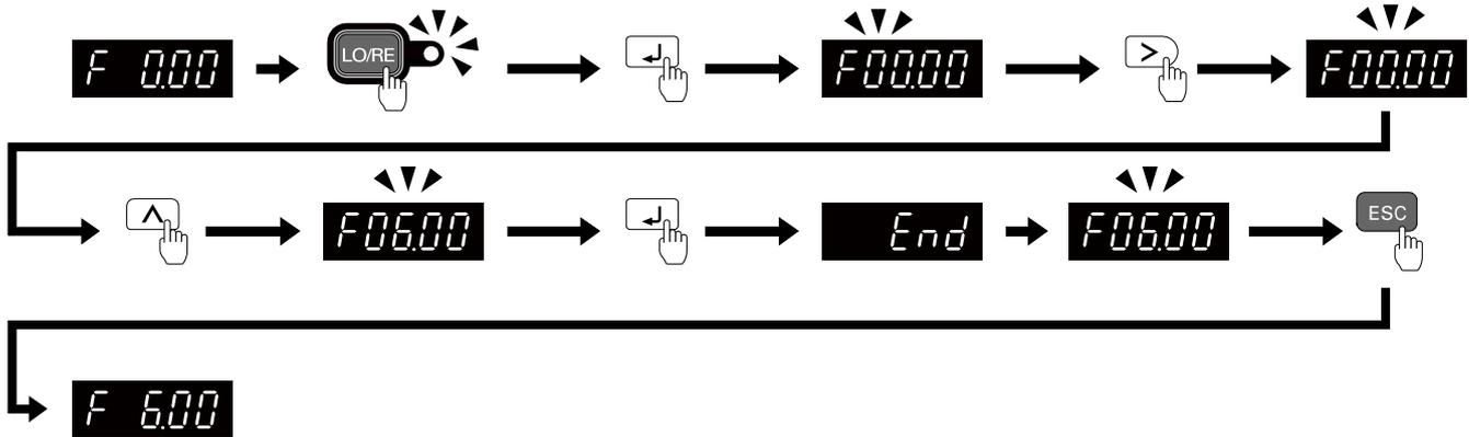
**Figure 4.7 Frequency Reference Setting in Drive Mode**
