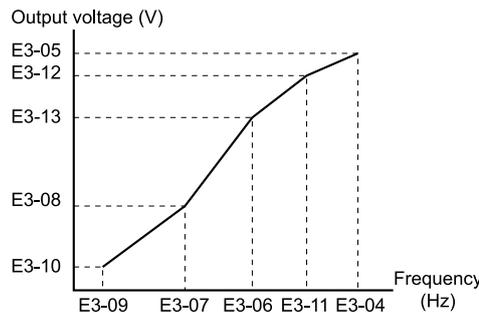
Figure 12.62 Motor 2 V/f Pattern Diagram
