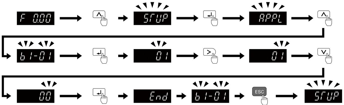
Figure 4.8 Key operation examples in Setup Mode
