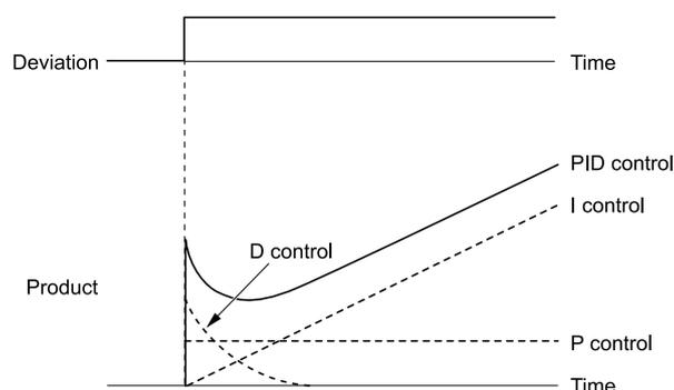
Figure 12.28 PID Control Operation
