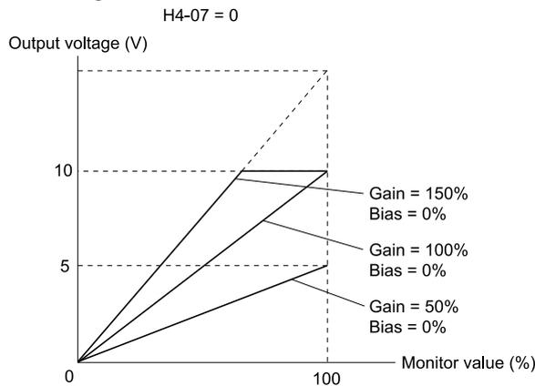
Figure 12.98 Analog Output Gain/Bias Configuration Example 1
