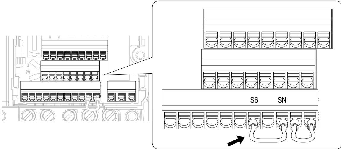
Figure 6.8 Self-Diagnostics Jumper Terminals
