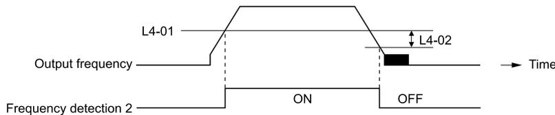
**Figure 12.1 Frequency Detection 2**
