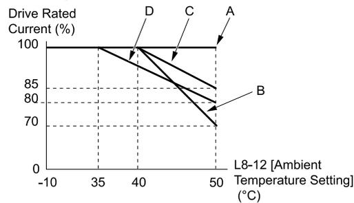
**A - L8-35 = 0 [IP20/UL Open Type] (0.5 m/s of airflow around the drive is necessary)**
