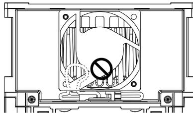
3. Put the cable and connector in the recess of the drive.
