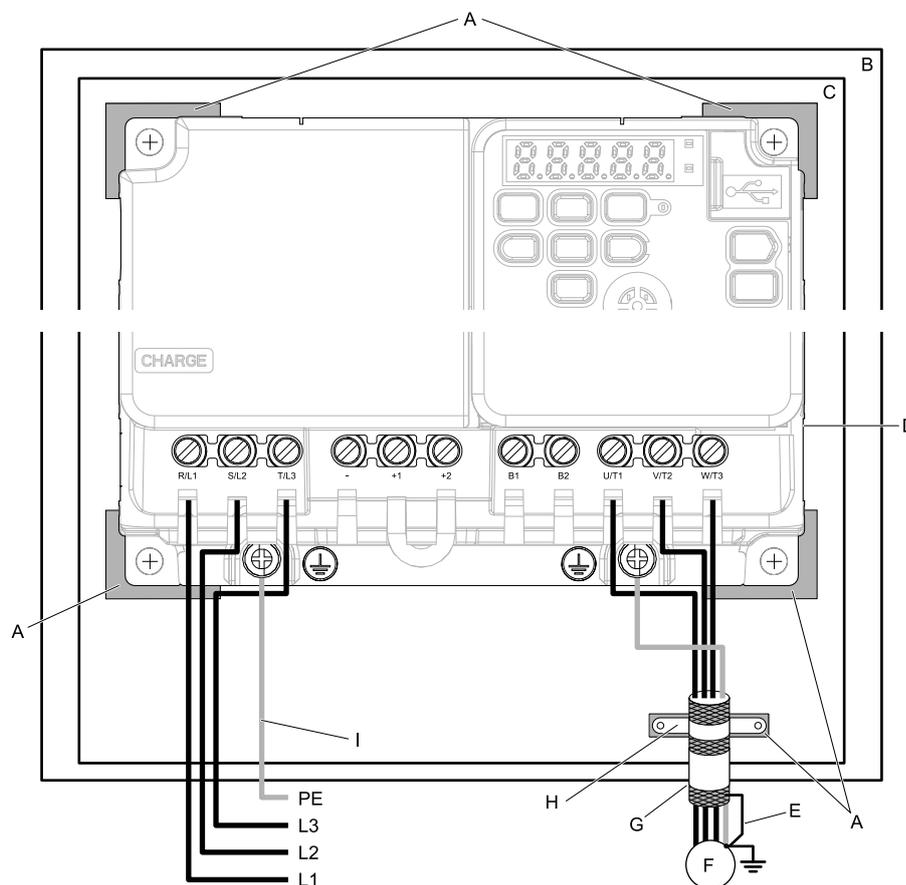
**A - Grounding surface (Remove any paint or sealant.)**
