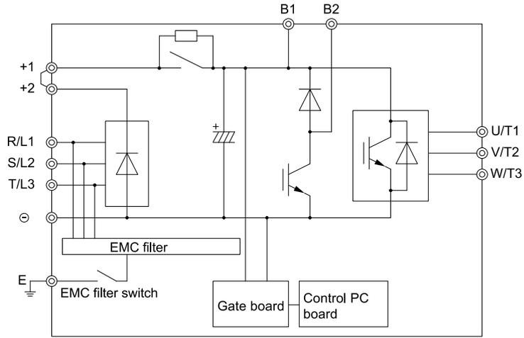
Figure 3.27 Drive Main Circuit Configuration 3
