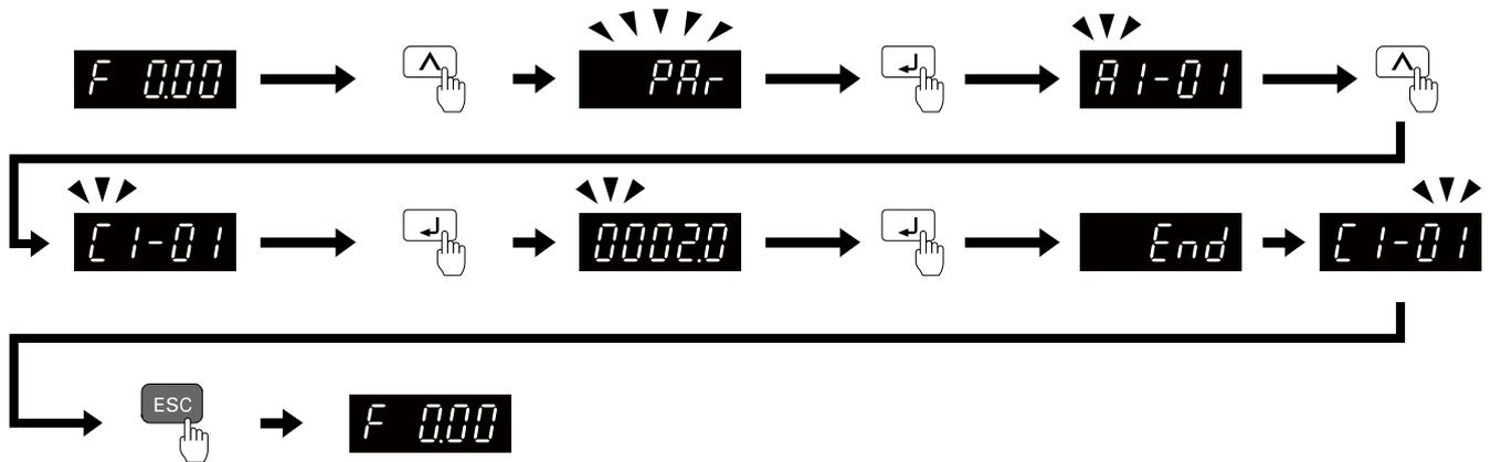
Figure 4.19 How to Change the Parameter Setting
