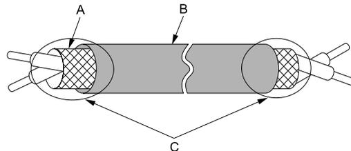
**A - Connect the shield to the ground terminal of the drive.**
