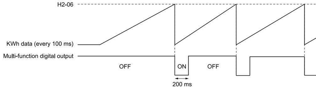
Figure 12.76 Example MFDO when Configured for Watt Hours
