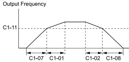
When the output frequency  $\geq$  C1-11, drive uses Accel/Decel Time 1 (C1-01, C1-02)
