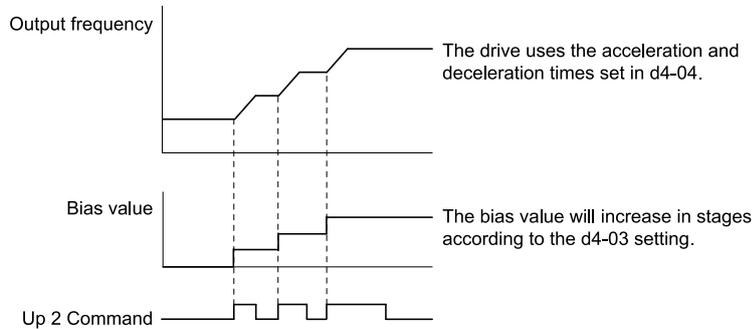
**Figure 12.57 Up/Down 2 Bias when d4-03 ≠ 0.00 Hz**
