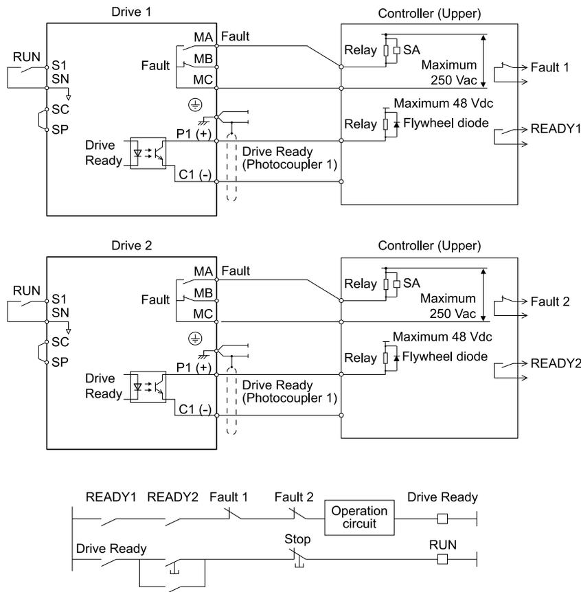
Figure 3.53 Interlock Circuit Example
