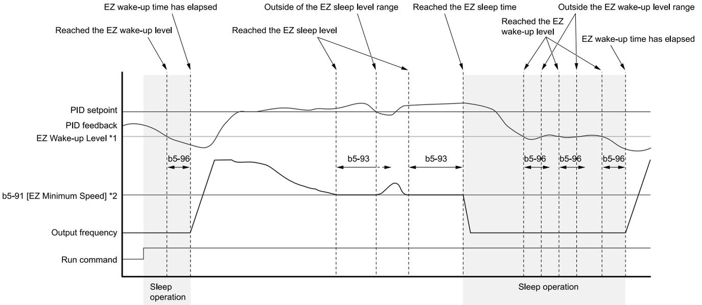
Figure 12.32 EZ Sleep/Wake-up Operation: PID Output is Normal and  $b5-92 = 0.0$  Hz
