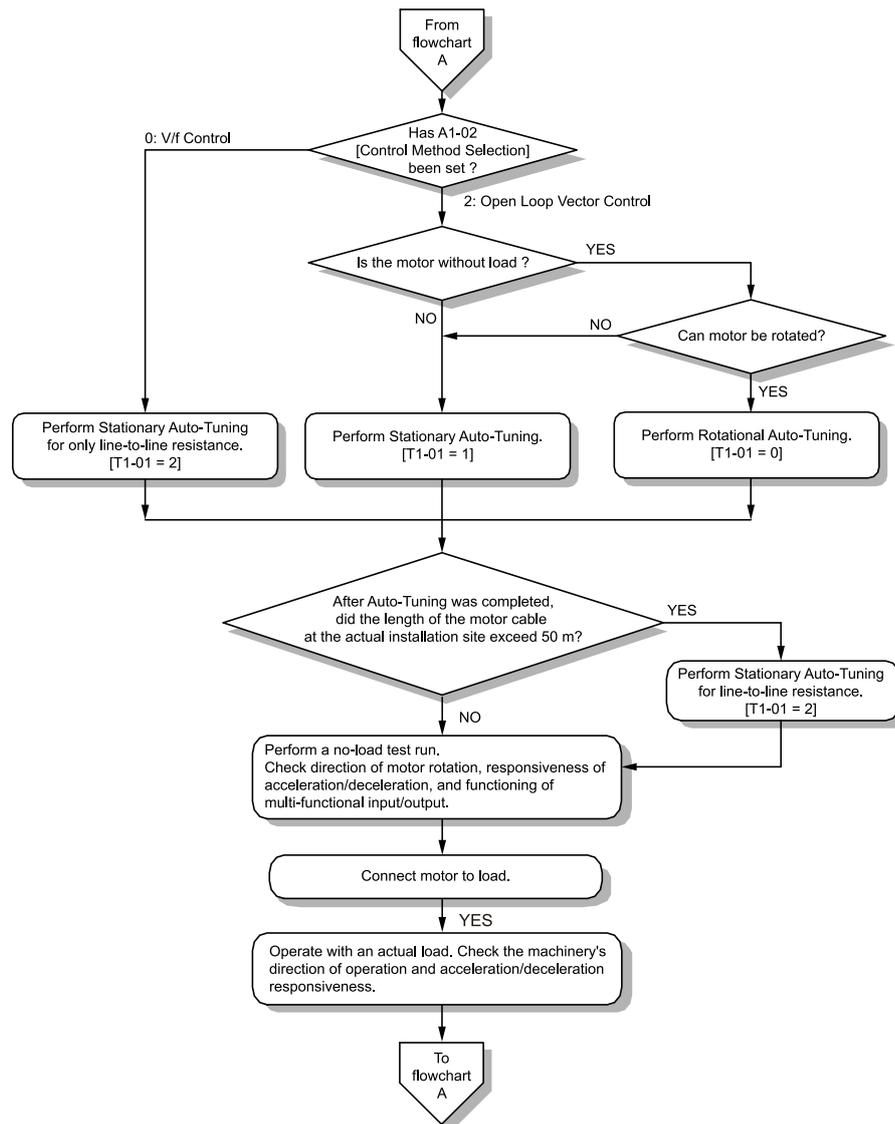
Figure 4.13 Induction Motor Auto-Tuning and Test Run Procedure
