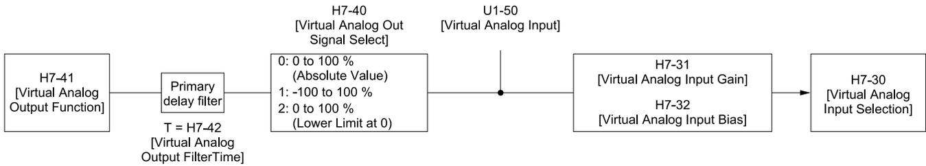
Figure 12.105 Virtual Analog I/O Functional Block Diagram
