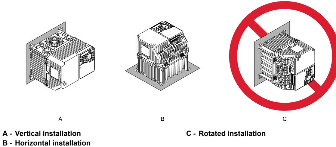
Figure 2.1 Installation Orientation
