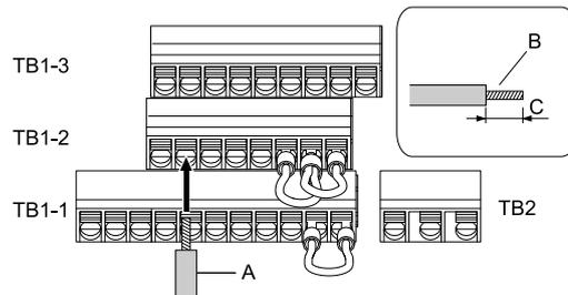
**A - Wire with a crimp ferrule attached, or unsoldered wire with the core wires lightly twisted**
