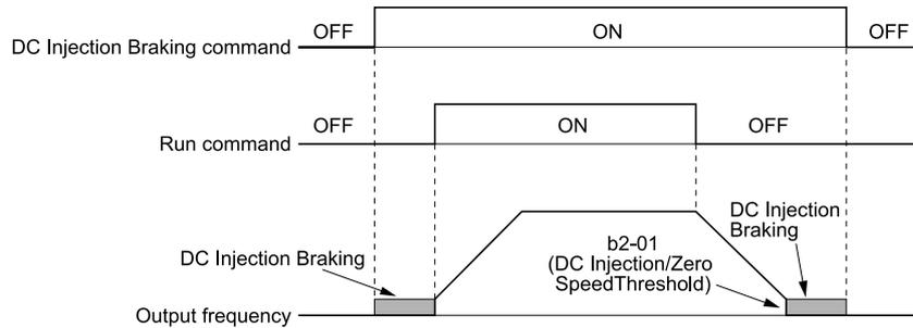
Figure 12.73 DC Injection Braking Time Chart
