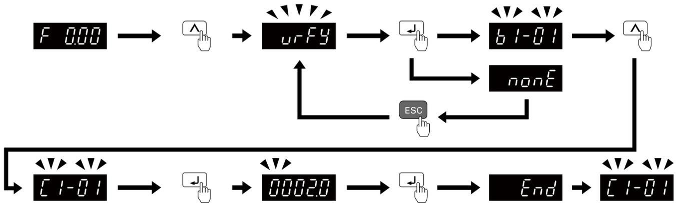
Figure 4.17 How to Examine the Changed Parameters
