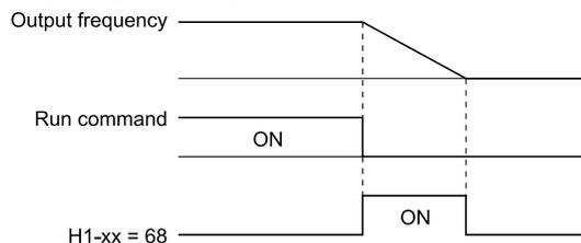
**Figure 12.132 High Slip Braking Time Chart**
