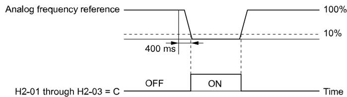
Figure 12.125 Detection of Frequency Reference Loss
