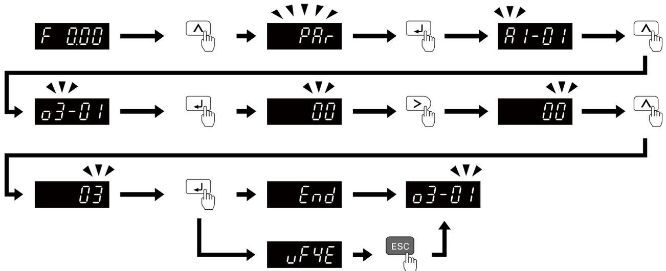
Figure 4.22 Verify Keypad Parameters and Drive Parameters
