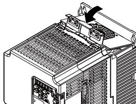
**Figure 8.15** Reattach the Fan Finger Guard
