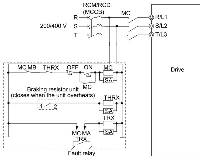
**Figure 3.56 Power Supply Interrupt for Overheat Protection Example**
