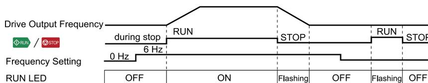
**Figure 4.4 Relation between RUN indicator and Drive Operation**
