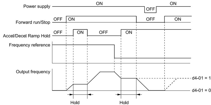
**Figure 12.53 Frequency Reference Hold with Accel/Decel Hold Function**
