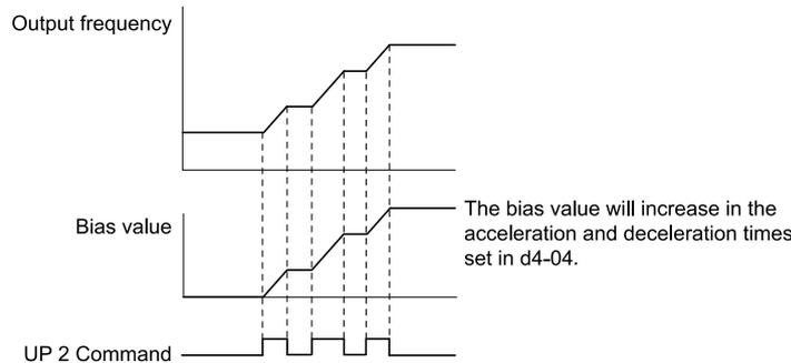
**Figure 12.56 Up/Down 2 Bias when d4-03 = 0.00 Hz**
