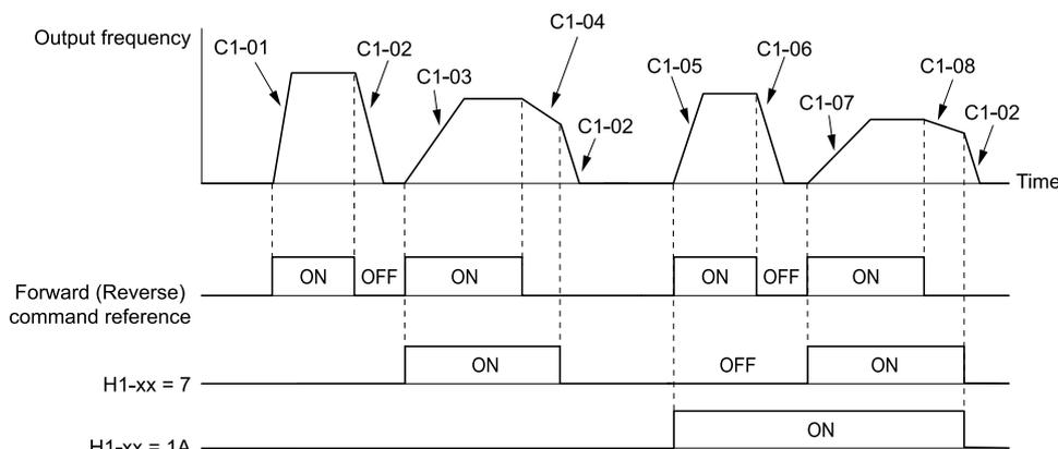
Figure 12.35 Timing Diagram of Acceleration and Deceleration Times
