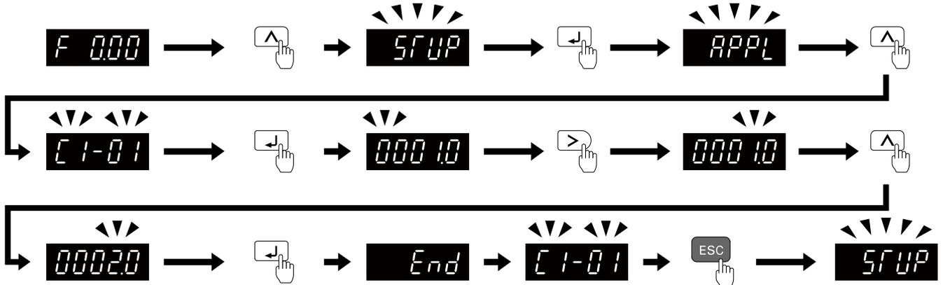
Figure 4.9 Key Operation Examples for Parameter Settings
